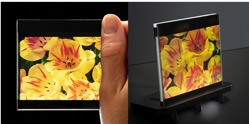
Figure 1. Ultra-narrow border organic LCD achieved by folding down the borders behind the display for the first time
