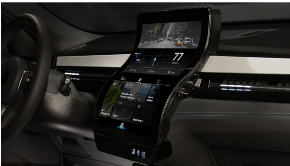
Figure 2. Example of two 12,1" curved OLCD displays, perfectly integrated into cockpit design and offering ideal and intuitive user interactions. Source: Novares
