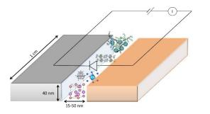
Figure 1. Schematic diagram of coplanar Au-Al asymmetric electrodes having a width of 1 cm, thickness of 40 nm and separated by a nanochannel (interelectrode distance) of 15-50 nm. Deposition of a suitable material in the nanogap and application of a bias between the electrodes allows current to flow from one metal to the other through the organic or inorganic material, that being the common underlying working principle of many electronic devices.
