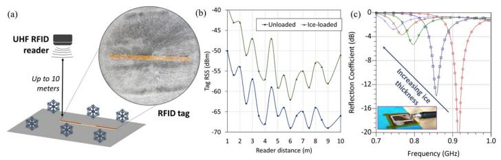
Figure 1. Robust large-area RF-enabled sensors for ice detection and monitoring in smart cities applications [1]: (a) illustration of the battery-free sensing system and a photograph of the ice-loaded RFID tag; (b) the measured sensor's performance showing at least 10 dB sensitivity; (c) the underlying operation principle where the ice "superstrate" shifts the resonant frequency; inset shows the dipole ice sensing antenna.
