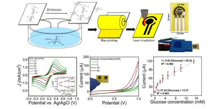
Fig.2. LIG on paper applied to electrochemical sensor production.
