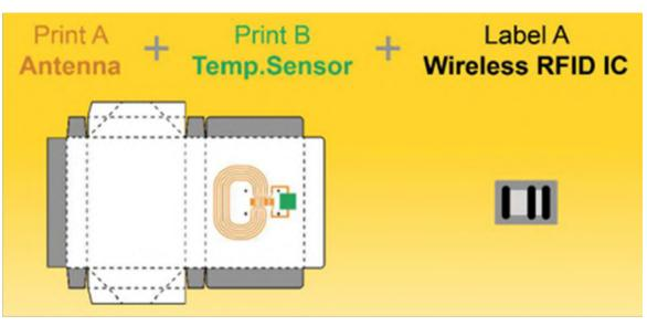
Components of a Temperature Threshold Indicator (TTI)
