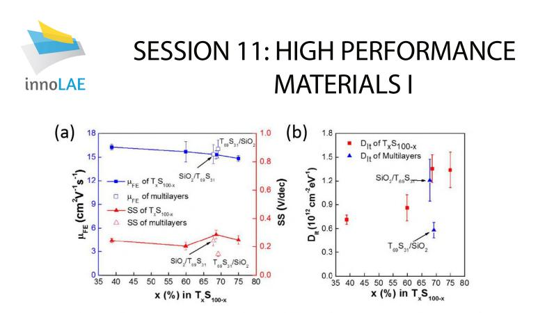
Figure 1 - (a) Field effect mobility and subthreshold slope and (b) trap density at the interface for TFTs employing the multicomponent and the multilayered dielectrics. Abbreviations: "T": T<sub>2</sub>O<sub>5</sub>, "S": SiO<sub>2</sub>.
