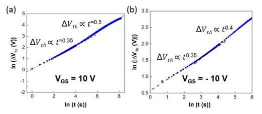
Figure 3 -  $V_{th}$  shift during (a) positive gate bias stress ( $V_{GS} = 10$  V) and (b) positive gate bias stress ( $V_{GS} = -10$  V) of a previously stressed device, showing power law time dependencies for both processes.
