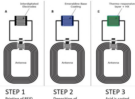
DIEP I Printing of RFID antenna and Interdigitated electrodes with silver ink SIEP 2 Deposition of Emeraldine Polyaniline base over interdigitated electrodes STEP 3 Acid is casted over polyaniline base turning into salt
