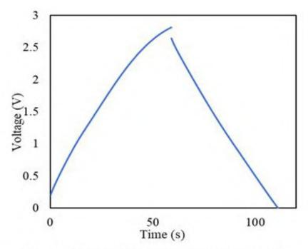
Fig. 3: Galvanostatic cycling tests (1 mA.cm<sup>-2</sup>)
