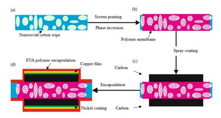
Fig. 1: Fabrication process of textile supercapacitor.
