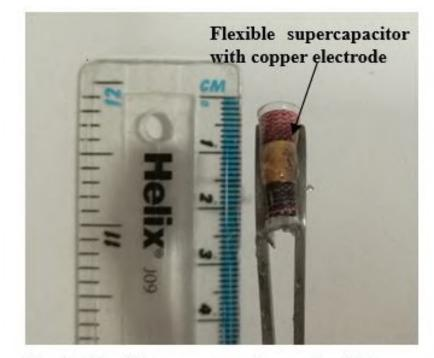
Fig. 2: Flexible supercapacitor under 180 degrees of bending conditions
