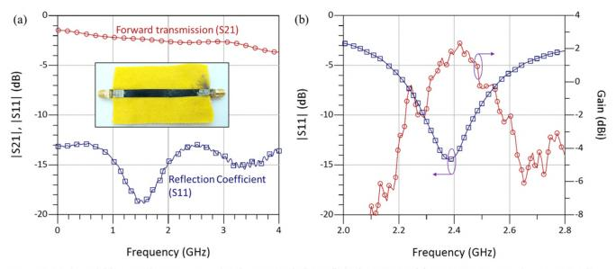
Figure 3. Biodegradable e-textile antennas and RF lines towards "green" chipless RF LAE: (a) A PEDOT:PSS printed transmission line for material characterisation and its measured transmission properties of the PEDOT:PSS line on a textile substrate; (b) The measured reflection coefficient and gain of a 2.4 GHz textile patch antenna using an all-polymer biodegradable radiating element.
