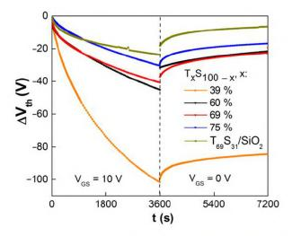
Figure 2 -  $V_{th}$  shift during positive gate bias stress ( $V_{GS} = 10 V$ ) and recovery ( $V_{GS} = 0 V$ ). Abbreviations: "T":  $T_2O_5$ , "S": SiO\_2.
