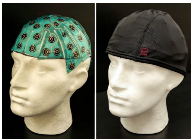
Figure 1: On the left model is the one-piece sensor array as it is formed around the head. On the right model is a production prototype of the covered sensor array that can be worn comfortably beneath a helmet.
