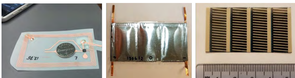
Figure 1. Temperature-logger with battery and supercapacitor and OPV replacing the battery
