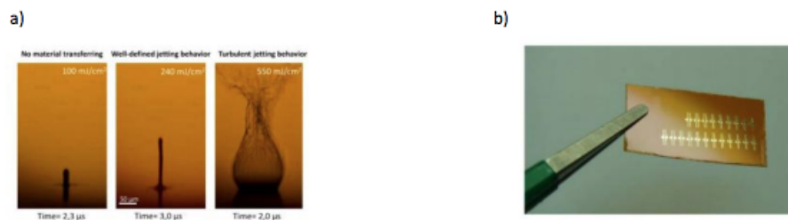
Figure 4: a) Printing type regime of Cu nanoink, b) laser printed Ag electrode pairs
