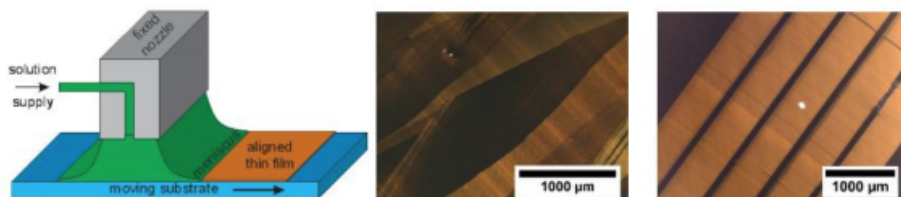
Figure 1: (a) Illustration of the zone casting setup. (b, c) Cross-polarized light microscopy images of the C 8 -BTBT single crystal without (b) and with (c) substrate patterning. The white arrow indicates the coating direction.
